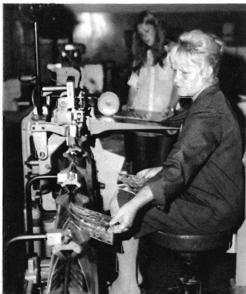
"Rail Ways" nearing completion, as Anja Jarvelainen operates the collating and stapling machine.
